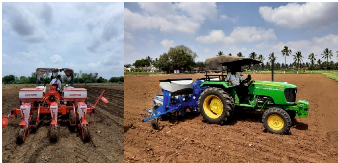
Planting of cotton using pneumatic planter
